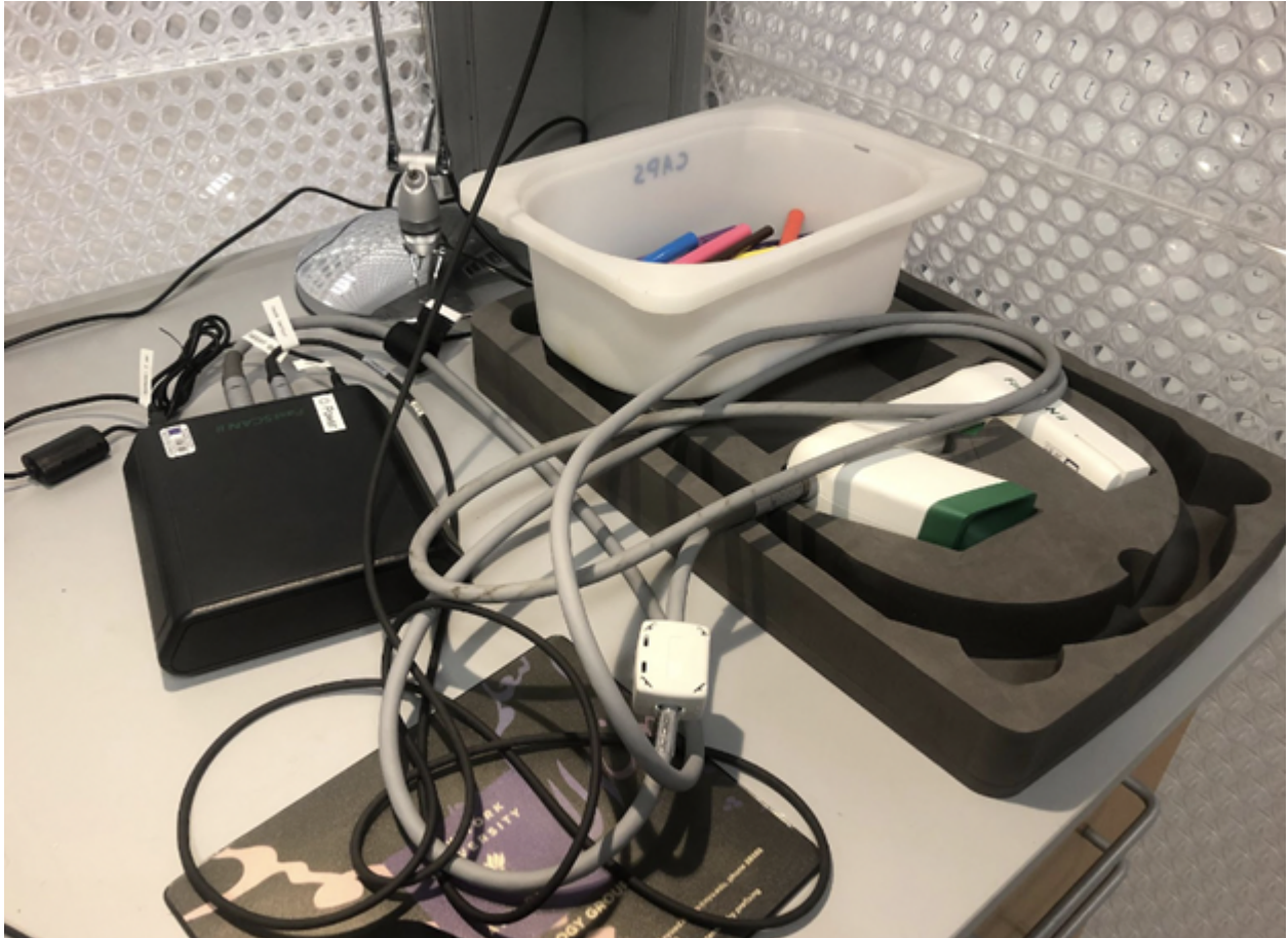
Fig. 23: FastScan should ALWAYS be placed like this: laser on foam, cables on table (not floor).
