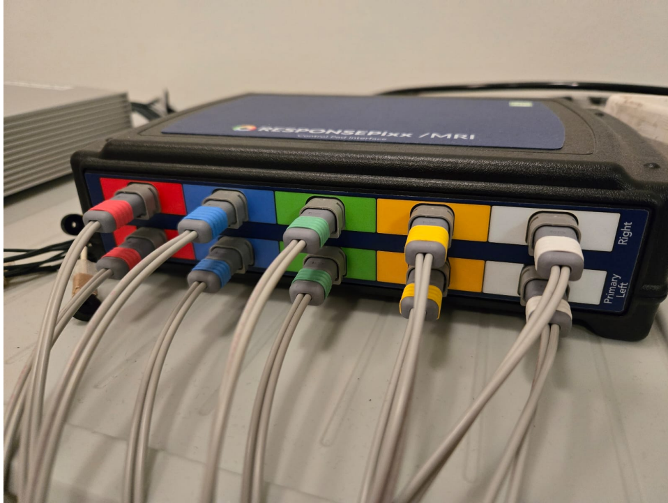
Fig. 10: Plugging the response box: Top row is the right response box, bottom row is the left response box .
